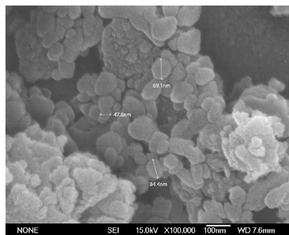
Fig. 5. Surface morphology of carbon nanoparticles obtained from heating of ZLHSA at 600 °C after acid washing process.
